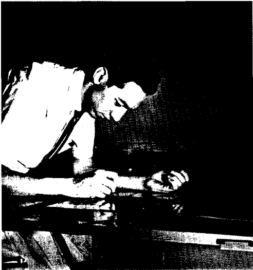
Mr. Schoon's main helper in the platemaking section is Charles Roemer. Here you see him preparing the negatives for the making of a plate. This happens to be a 16-page section of The PLAIN TRUTH . First, he carefully covers any scratches or holes there may be in the negatives with a black paint. This is called opaqueing , because what the process does is to keep light from passing through the negative wherever it is applied, making it opaque. Next, Charles lays the complete section of negatives on a frame over a light-sensitive metal plate, and locks it into position. The last picture shows the powerful arc light burning through the negative and forming an impression on the plate.
